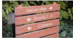
These wayfinding signs are constructed in a way where each sign can be slid out the top of the sign, this enables re-ordering or updating of the sign without re-installing a whole new sign in the eventuality there are layout or name changes to the property.
