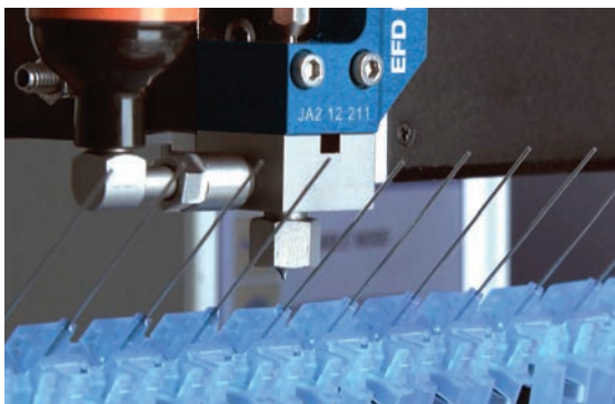
A pneumatic jetting system, the Liquidyn® P-Jet valve applies micro-deposits as small as 3 nL.
