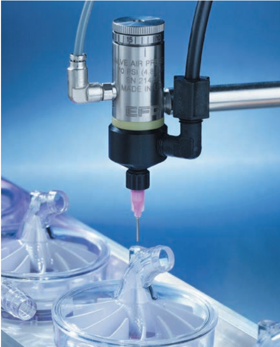
A 752 valve applies UV-cure adhesive to a medical pump.
