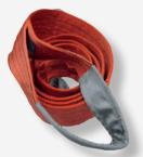
Superior quality 5 Tonne Duplex Webbing Sling Manufactured to BSEN 1492-1:200 from Mudfords. With a 7:1 SWL ratio, this is the perfect lifting accessory.
