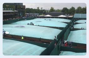
We produce the Inflatable Tennis Court Covers used at the Wimbledon Tennis Championships. They are made of a lightweight material which, once rolled out across the court, are inflated by fans to form a dome allowing water to drain into channels around the court.
