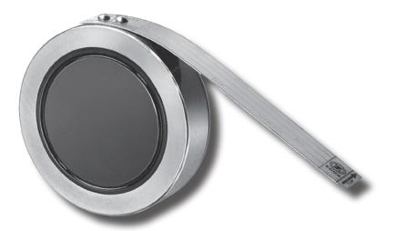
ZOOK's new Fluoropolymer Sintered Graphite Rupture Disk offers enhanced features when compared to resin impregnated graphite disks. The Fluoropolymer coating is sintered at a high temperature onto a graphite blank. The durable coating seals the graphite material enhancing the corrosive capability and allows the disk to operate at sub-zero to elevated temperatures with minimal effect on the burst performance of the rupture disk.
