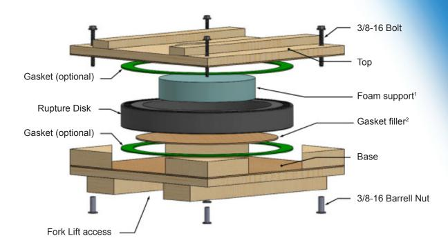
Disks rated with burst pressures less than 15 psig and without a vacuum support will be supplied with a foam membrane support.
