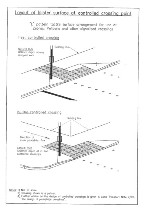
Figure 4: Layout of blister surface at controlled crossing where the back of the edge of the tactile is not parallel to the kerb.
