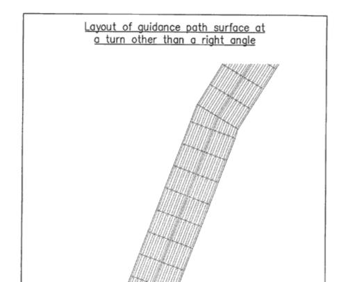
Guidance on the use of tactile paving surfaces
