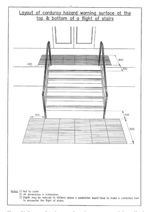
Figure 21: Layout of corduroy surface where ramp access is immediately adjacent to steps
