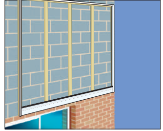
3. Fit first plank at base
