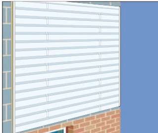
5. Ideal joint design when using individual butt joints.
