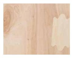
Generally as BB grade but with the possibility of a greater number of repairs, open defects and discolouration. This grade can also arise from the rejects of higher grades. Suitable for applications where a strong, stable core is needed but where it is accepted the face quality can vary.
