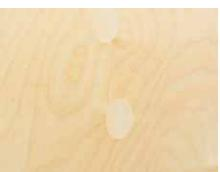
Mainly solid veneers with only small repaired veneer splits and pin knots allowed. Larger open knots are repaired with wooden plugs/ patches. The shape of the plug repair can be described as 'oval' or 'butterfly' dependant on manufacturer and the number of repairs is limited to eight per square metre. Some solid light and dark knots are admissible.
