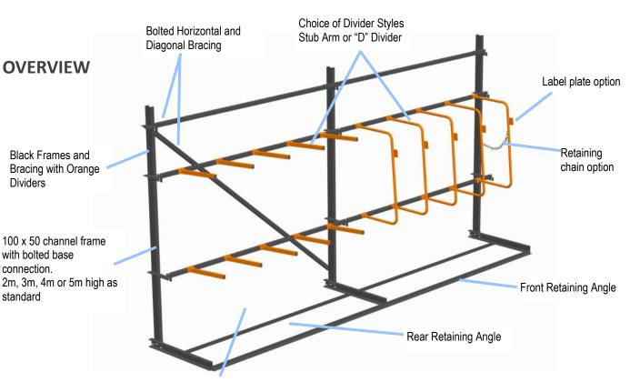
Standard Bay Width of 3m with "make-up" bays to suit run lengths
