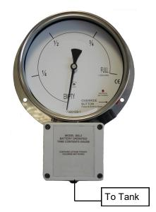
RESET BUTTON - In the unlikely event that you think the reading is incorrect, the reset button facility can be operated, this forces a reset of the timer system. When the button is pressed and released, the reading will rise then fall slightly, allow to settle, reading can now be taken. Once RESET has been used, it cannot be reused for a minimum of 30 mins. Please note that this operation will dramatically reduce the battery life.
