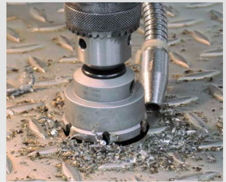
Drilling in checker sheet
