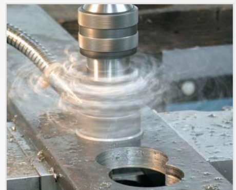
Drilling in flat steel
