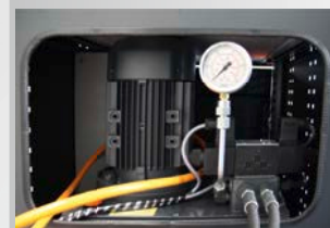
Dual-circuit hydraulic unit in cabinet base
