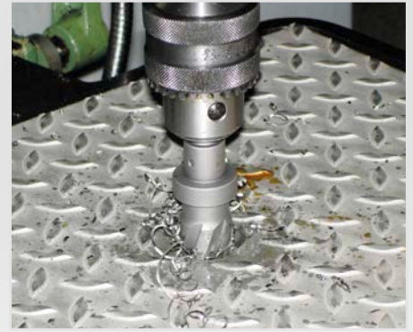
Drilling structured sheet metals
