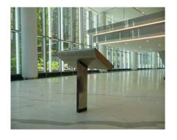
The outcome of this design is a completely customized table top touch screen to the specification given by Velvet Principle. We used one of our own POS-Line displays manufactured in Germany in a size of 42". This POS-Line unit has PCAP dual touch, edge to edge technology giving the screen a true-flat look and has a brightness of 700 CD. The unit also includes an aerofoil shaped free-standing leg and is fully fabricated in brushed satin stainless steel.
