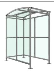
The Badby shelter is a free-standing, open sided shelter designed for on site assembly, constructed from galvanised mild steel. Complete with a 4mm PETG clear sheet roof, and side panels. Front-to-back curved roof.
