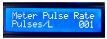
The system is set for a meter with a 1 pulse per Litre output
