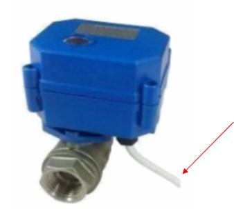
The 230VAC supply to the valves is generated from within the alarm unit. 15 to 25mm valves are supplied with a red and black cable whilst larger valves are red and green. For good practice connect live to the red wire and neutral to the black or green wire.
