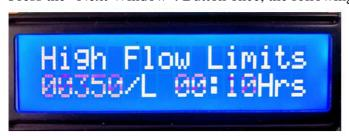
High Flow ALARM limits, the total Number of Litres over what period of time. i.e., 350/L 00:10Hrs, if the unit sees 350 litres within 9 minutes the unit will go into alarm
