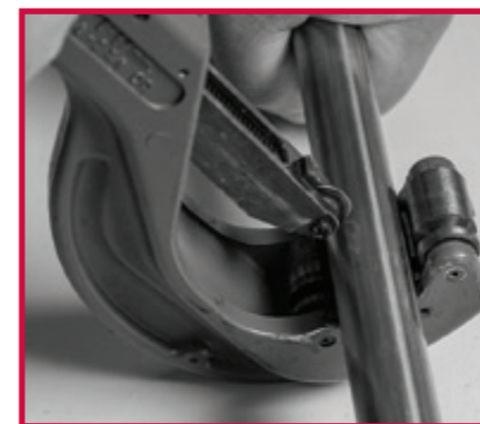
1. Cut tube at right angles to length.
