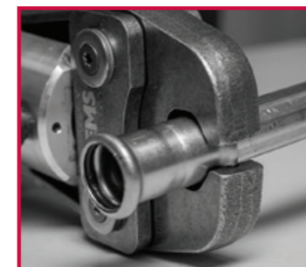
5. Place the correct press fitting jaw into the machine and insert the fastening bolt. Open the jaw at right angles to the fitting and activate the machine to pressfit.
