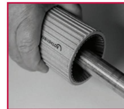
2. Deburr tube both internally and externally to prevent damage to the fitting seal on assembly.
