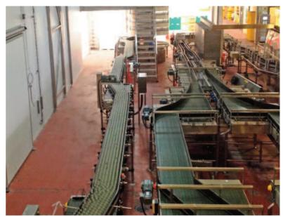
Caption: Colwall Conveyor Systems re-planned and moved an existing production line in order to create a 2m forklift truck access between the equipment and a new partitioning wall at Britvic.
