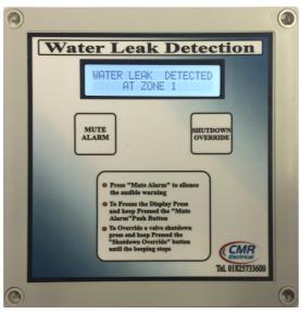
The LD4-2 range has been designed to monitor four independent zones in critical areas for water leaks via linier detection cables or spot sensors. Any number of spot sensors or a maximum of 50 metres of linier water detection cable can be connected to each zone.
