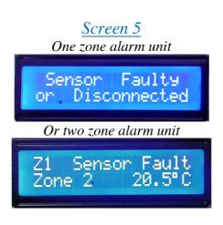
The sensor on zone 1 has become disconnected or is faulty
