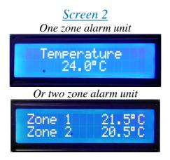
The unit has no alarms and is showing the temperature in each area
