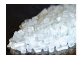
Silane modified polyolefin (POR) adhesives are often used in place of PUR adhesives when the bonding surfaces pose a challenge for PUR. For instance, polypropylene surfaces which is common in automotive assembly. POR hot melts are also much more environmentally friendly (do not contain isocyanates). POR applications include seats, carpets, foam-based materials, cable attachment, bonding door sill protectors, gear knobs, and emblems.
