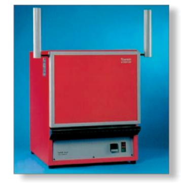
The heated chamber is formed from hardwearing sillimanite and is located within the one piece outer case, an air gap and a graded selection of the latest high efficiency lightweight insulation between chamber and case achieves both a high thermal efficiency and cool outer case.
