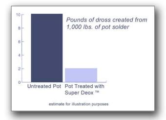
Super Deox is specifically formulated to reduce and prevent the oxides of solder, (known as dross) on still pots and wave solder machines. Super Deox is a white powder material that will lower your cost by reducing dross and solder consumptions.
