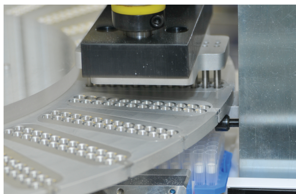
Automated filter assembly, no human contact
