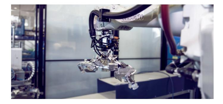
When the German company FRIMO established a plant for gluing interior fittings for the car industry, the opportunity to fully utilize its robots' mobility was decisive. Equally significant was the capacity to automatically change tools with precision and maintained function. The choice fell on the swivel tool changer from Robot System Products.
