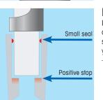
Low force tip ejectionRainingLTS models reduce tip ejection forceson thedramatically. LTS tips incorporate a smallreducesealing area and a positive stop that letsand syou know exactly when the seal is madePipet-
