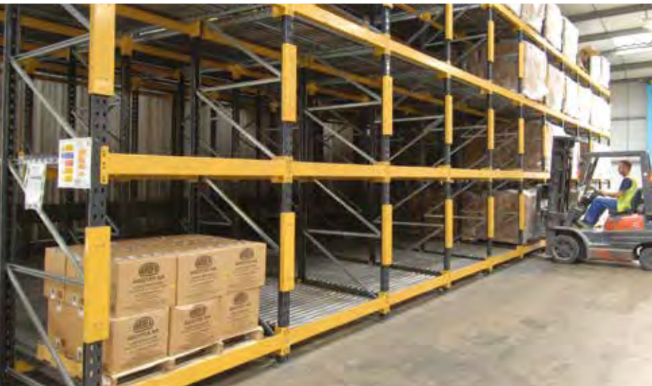
Pallets are loaded onto wheeled carts or rollers and are pushed back along inclined beds. When a load is retrieved the remaining pallets roll forward into position at the picking face.
