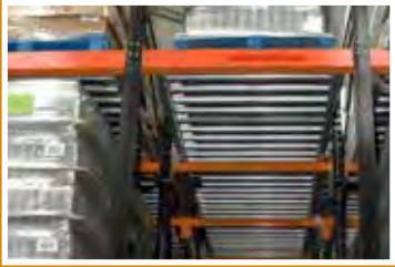
Full width roller accepts mixed pallet sizes and can accommodate up to 10 pallets deep.
