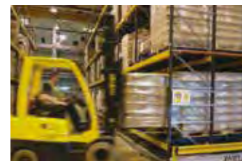
Pallets are loaded onto wheeled carts or rollers and are pushed back along inclined beds. When a load is retrieved the remaining pallets roll forward into position at the picking face.
