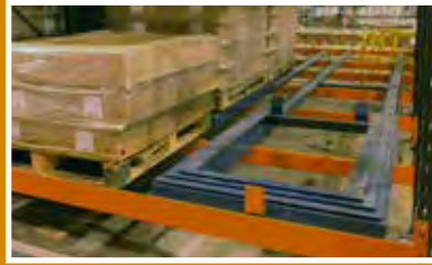
Carts interlock to prevent jamming and to control pallet descent. Accommodates up to w6 pallets deep.
