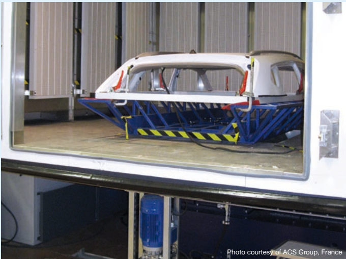
Combined climatic and vibration testing of car sunroofs
