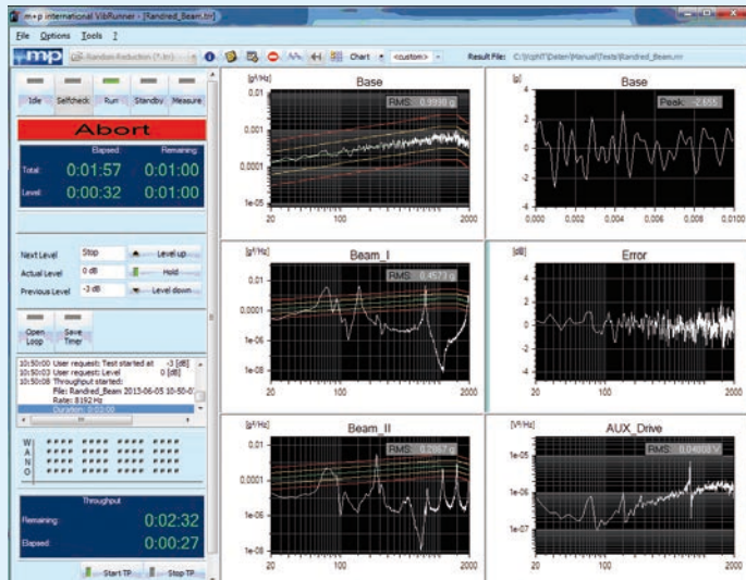
Online random data reduction with throughput to disc recording
