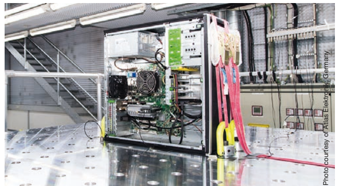
Vibration testing of a PC
