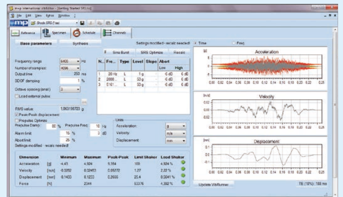
Setting up a shock response spectrum (SRS) test
