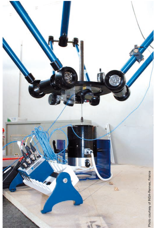
Modal analysis on a parallel robot
