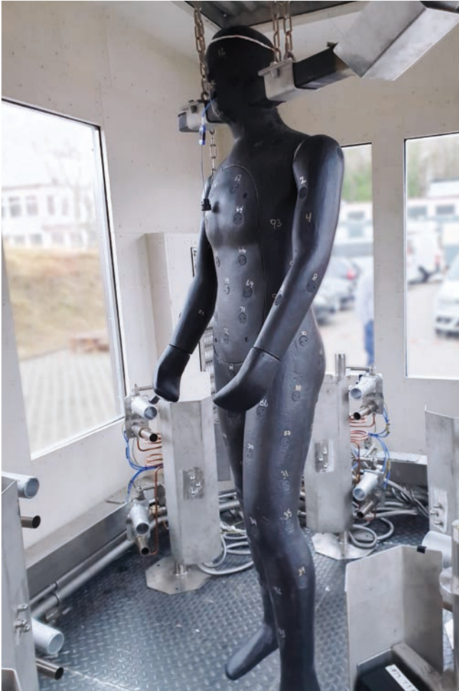
Thermo-Man® mannequin equipped with 122 heat sensors
