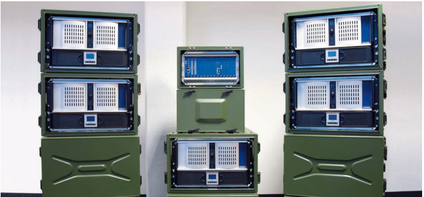
Mix of Spectrum PCI Express cards and m+p VibMobile front-ends in shock-isolated, vapour-proof boxes
