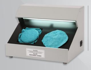
VeriVide are pleased to announce the launch of their new Pilling Assessment Viewer (PAV) for the textile market. This new PAV unit has been developed in conjunction with Technicare Services Ltd, and in accordance to EN ISO 12945 standards incorporating all 3 parts and adopting the following test methods...
