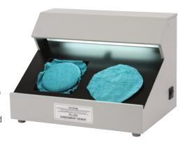
All VeriVide Textile Texting products incorporate high frequency electronic ballasts for instant flicker-free illumination and silent operation.
