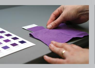
Colour requirements for manufacture and retail are complex and diverse. To ensure product colour, several types of light source are used (e.g. Artificial Daylight and a Point of Sale Light). Multiple light sources are also necessary to reveal colour inconsistencies and metamerism.
