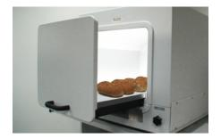
Samples to be measured for colour are in the DigiEye Cube, which excludes ambient light in favour of controlled, consistent lighting to CIE D65 standards. Different illumination geometries are possible, including angled and diffuse lighting.
