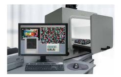
Samples to be measured for colour or appearance are placed on a neutral grey background in the DigiEye Cube, which excludes ambient light in favour of controlled, consistent lighting to CIE D65 standard. Different illumination geometries are possible, including angled and diffused lighting options.
