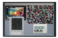
DigiEye software relays data to a calibrated monitor and printer for instant comparison and, if needed, colour-accurate printing of images for use as master product standards.
