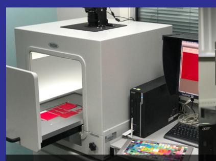
Imaging of samples either at supplier or sourcing office via the VeriVide DigiEye system
