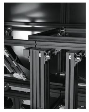
The measurement chambers must be completely enclosed and blacked out for the use of 3D camera systems. The products to be inspected are to be transferred to the chamber using AGV systems and fed in automatically. Inside the chamber, they are to be separated, photographed and weighed on individual measuring stations.
