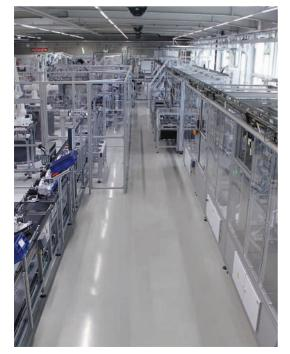
Fully automatic assembly line for suction pipe modules that is approximately 45 metres long, equipped with guarding including protective fences and machine housings. Passages and transitions for system maintenance also have to be created.
