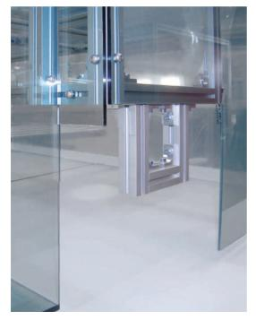
A hood for extracting dust particles is required for the production of electronic parts. The contour as well as the inputs and outputs are specified by the customer. The hood must be equipped with a suction nozzle for an extraction system provided by the customer. The circulating dust must not produce electrostatic discharge. The housing needs to be transparent but must also block UV radiation.
