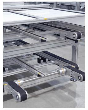
A cooling and curing section is required for a battery production line. The section must be able to process loads of up to 1700 kg on the upper line and 1000 kg on the lower one, of which up to 500 kg is for accumulated operation.
