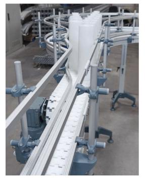
Cooling line for plastic bottles. The bottles are ejected from the blow moulding machine in two lines and must then be converged on a conveyor line for feeding to the subsequent cutting machine and inspection. The bottles must be transported upright.
