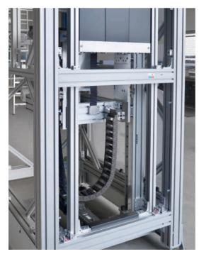
A solution with interlinking across multiple levels and processing stations is required for the production of electric motors. Lifts for lifting, lowering and turning are used to transport the pallets to the various levels and align them. The total load per pallet is about 100 kg per pallet over an area of 500 x 500 mm.
