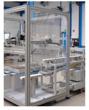
For use with our innovative and reusable small load trays known as IKLTs, the customer requires a low-cost automation solution with semi-automatic transfer and an automatic unit for stacking and unstacking the trays from the base of the transport box.
