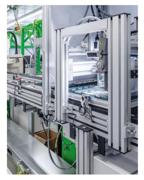
System for producing digital antibody tests. Because sensitive electronic components are used in the tests, the entire system will be located in an ESD protection zone.
