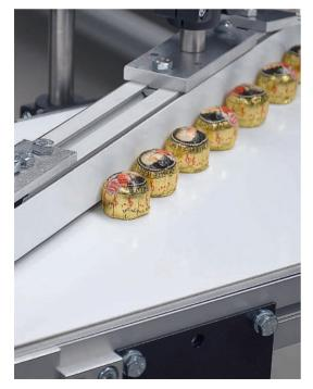
In a confectionery production department, packaged chocolates need to be separated upon exiting the individual packaging unit and conveyed to the repackaging process. The conveyor unit needs to be mobile in design so that it can be used on different production lines. In addition, the parts of the unit that come into contact with the product must meet the hygiene standards for transporting foodstuffs.
