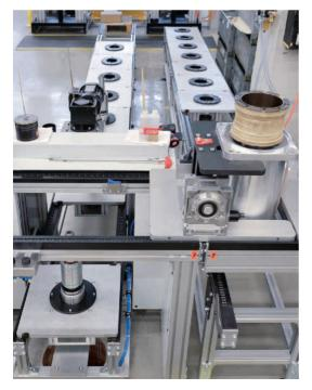
Semi-automated workstation interlinking of rotating assemblies for stretching synthetic fibres. The solution required was an interlink between the shop floor press, marriage station and electrical testing station that was optimally adapted to the space from a logistical perspective.
