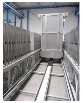
Planning, design and construction of an automated system line for researching root growth in plants. The plant packs are to be automatically swivelled to take repeated photographs of them in a darkened enclosure. It also has to be possible to remove them individually. Process reliability is required to ensure the research results are valid.
