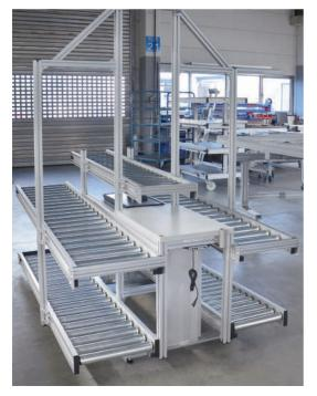
Workbenches for assembling wireless mobile phone charging cradles. The workbenches must be individually adapted to the respective work steps. Furthermore, they require a feeding and removal system to keep conveying times to a minimum. The workbenches must be designed with full ESD protection.
