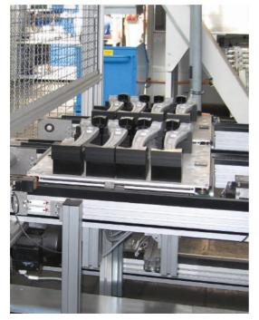
In the production of longitudinal and cross beams, the production systems, the packaging robots and a station for manual tasks need to be interlinked.
