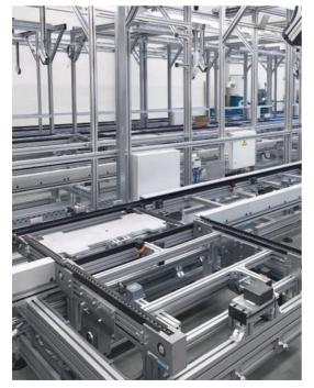
An operation installing car seats requires a circulation system where workers can fit and process the seats.
