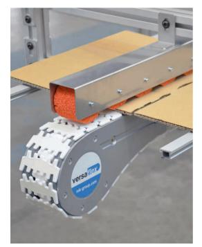
Unfolded shoe boxes first need to be sprayed with adhesive and then folded in the next machine in a packaging plant.
