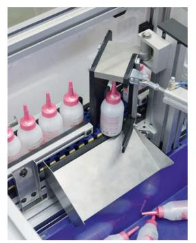
An operation producing cosmetics bottles requires the interlinking of two machines. The bottles need to be transported around a 90° curve. When the product is changed, the bottles are to be discharged so that the interlink can run to empty. The interlink must be able to transport different formats.
