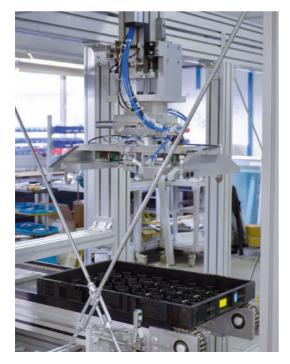
The customer required a palletiser with a tray recirculation system: Pallet trucks are used to feed Euro pallets loaded with trays into the system using an index station and then remove them again at the end of the process. The palletiser destacks filled trays from the pallets and feeds them into the recirculation system. The system needs to be able to recognise and handle different tray types and different stack heights on the pallets.
