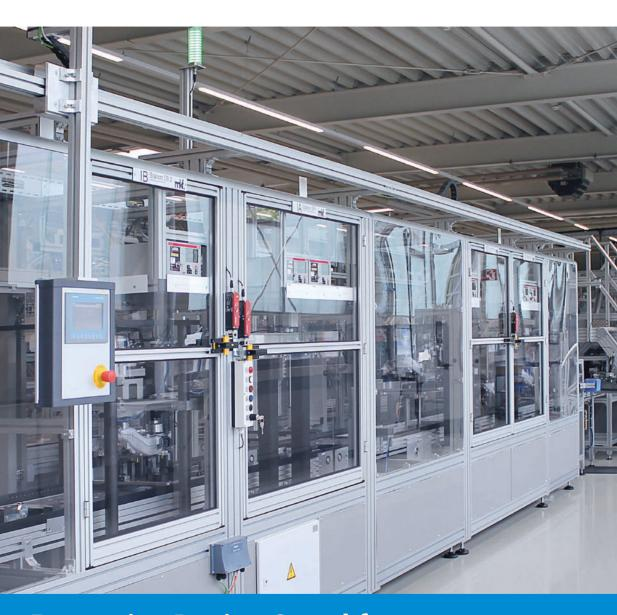
Protective Device Guard for 45-metre Long Assembly System
