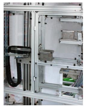
A solution is needed to interlink lathes in a production process for titanium screws with thread whirling machines. The following functions are required for the baskets: lifting/lowering, guided conveying, positioning, gripping, tipping and buffering. The system must be fully automated and be able to operate autonomously for at least one shift.
