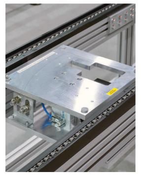
A horizontal pallet circulation system was needed for the production of electric motors for an electric SUV. The workpiece and pallet weigh about 100 kg, which means a total load of 160 kg per meter of conveying path.
