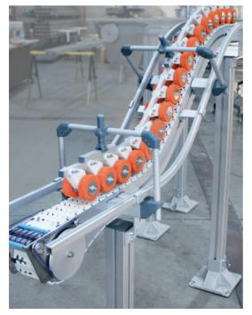
Only a very limited amount of space is available for a solution to transport chocolate bars. A height difference of around 480 mm and a 90° curve must be circumnavigated. During the vertical ascent, the chocolate bars must not slide backward even when the conveyor is stopped.
