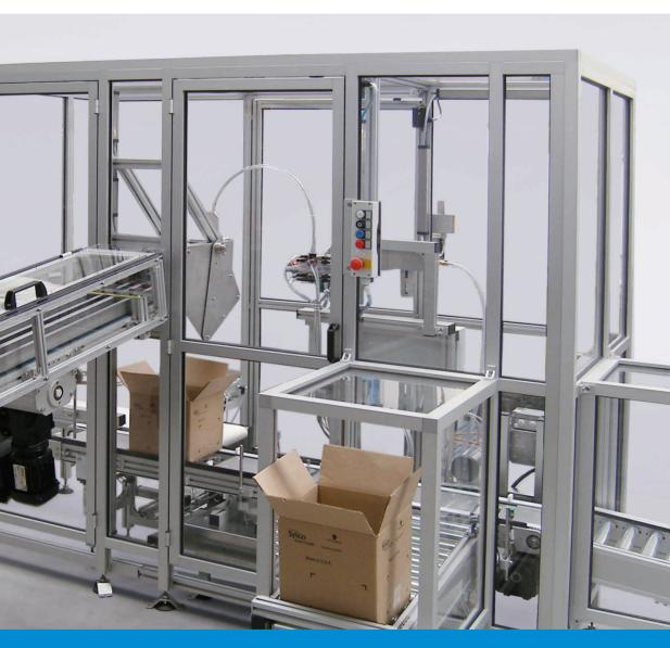
**Complete System for Filling Cardboard Boxes** with High-level Hygiene Requirements
