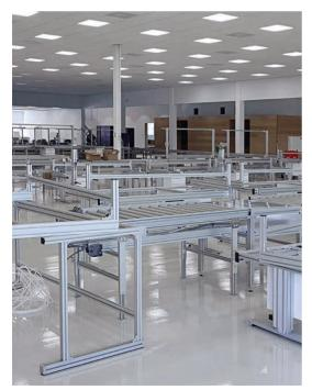
Assembly line with 10 workstations where workers have to install and check analysis units, connected via a conveying path. In order to support lean production and reduce the burden on employees, it is important that the workstations are designed to be as ergonomic as possible. Since the products to be assembled are very sensitive to ESD (electrostatic discharge), the workstations must also feature ESD protection.
