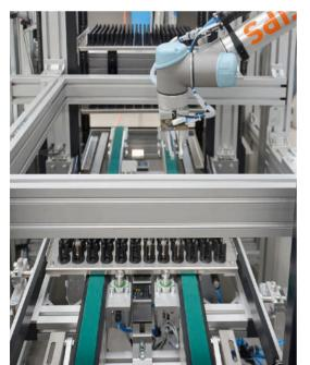
A system is required where trays for steel turned parts are loaded and unloaded fully automatically. The trays are to be buffered upstream and downstream from the palletising station for further automation. Once the first buffer store is manually filled by a worker, the system should be able to operate completely automatically.
