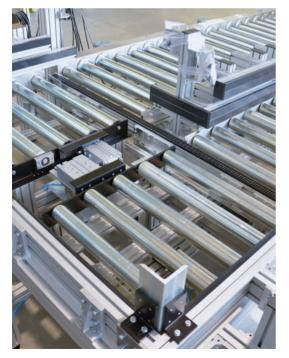
A solution for transporting standardised plastic euro pallets to and from a production system.
