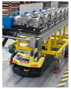
A flexible solution for conveying components for the assembly of motors is required. There is no interim storage on the assembly line, meaning that production occurs just in time. Zones for walking and driving must remain clear with a relatively low flow rate.
