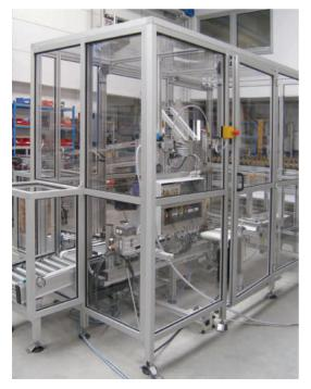
Design and creation of a carton filling machine for different tube shapes in the cosmetics industry. Interlinking of carton erectors, from filling to further packaging.
