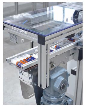
The labelling and packaging machines in a food supplement production line are to be interlinked with each other. The bottles need to be transported around a 90° curve and separated on the line so that the appropriate number of them can be packaged in cardboard boxes. Manual packaging should also be possible without any major refitting measures.
