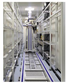
Storage of various transport containers over several levels. The boxes have to be put away in accordance with the cleanroom class ISO-4.
