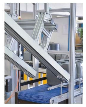
Upright plastic canisters have to be interlinked with each other through two processing stations. The required interlinking crosses a walkway and track.
