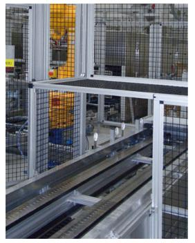
Interlinking multiple work stations with different cycle and changeover times. Large dishwasher casings need to be stopped for visual inspections and to assemble additional components. The conveyor technology must be designed in such a way that the casings can be transported safely and at the same time removed easily by workers.
