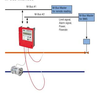
The M-Bus has established itself as the standard for meter reading as it has been standardised in EN 13757, and offers a variety of other features. Advantages include:
