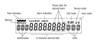
The multi-function display shows the eight-digit meter reading, along with symbols and short texts for user operation purposes.
