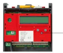
Under the cover, and thus protected by the lead seal, is the Service button, which allows additional service information to be displayed and adjustments to be carried out.
