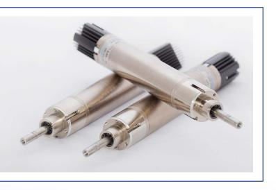
Strokes range from 5mm to 250mm and peak forces up to 600N are available. All models are provided with closed loop position feedback by non-contact linear encoders with resolution options ranging from 5 microns to 5 nanometres. The direct drive nature of their linear motor completely eliminates backlash and assures excellent repeatability.
