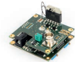
Fig. 8.s: OEM amplifier board for driving magnetic actuators
