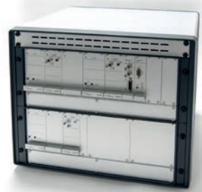
Fig. 8.o: Rack cabinet mounted LA75C push pull amplifier channels for driving large capacitance piezo mechanism
