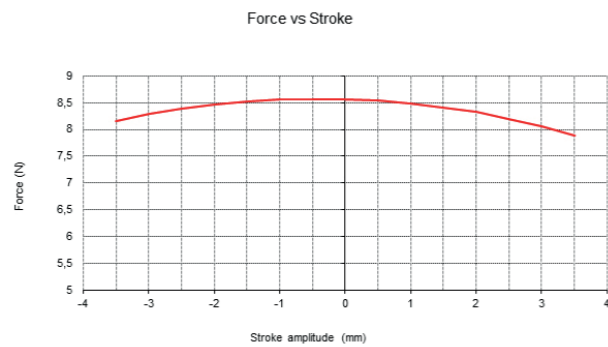
Fig. 2.z: Moving coil linearity of force versus stroke
