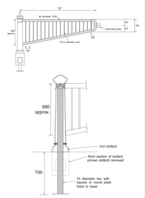
With this design of gate no hinges are used. The bollard pivots around a solid steel core specially constructed within the confines of the bollard.
