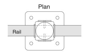
Pass the rail through the post to the desired position. Drill through opposite sides of the railing post and tube to receive two 6 or 8mm diameter steel pins (optional extra) drifted below the surface. Fill the resultant holes and the gap around the tube with an adhesive sealant (optional extra), then dress flat and touch-up paintwork to match surround.
