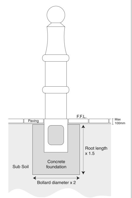
Bollards should always be securely fixed in 3:2:1 concrete mix, sulphate resisting if necessary. Certain sites, (dependant upon location) may require a quick setting concrete to be used.
