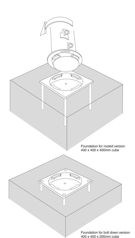
This type of socket has a separate cover plate for use should the bollard be removed for any length of time. The cover plate should be stored independently from the bollard.
