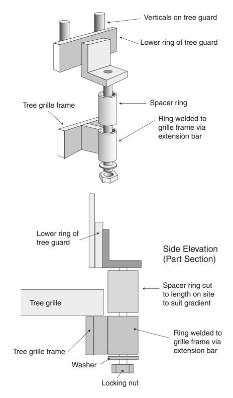
The tree guard/frame will accommodate three to four of these brackets depending on the design of the grille and guard. All components are provided if a frame fixed guard is ordered.
