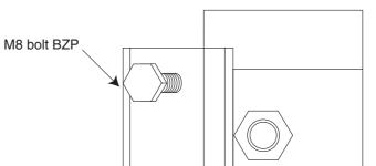
This is fabricated in 8mm mild steel with BZP threaded bar & bolts in a single colour gloss finish.
