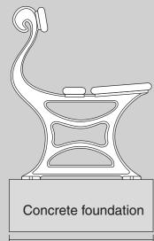
Foundation per seat end length = product depth + 150mm width = 300mm
