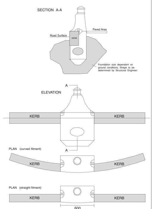
Bollard 193 has been designed to deflect lorry trailer wheels, thus preventing them from mounting kerbs and damaging railings or pedestrians.
