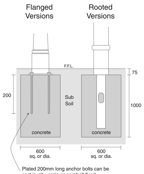
cast in-situ, resin or parabolt fixed.
