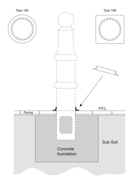
Loose fit cover plate prior to installation of bollard if superstructure does not allow post-installation fitment.
