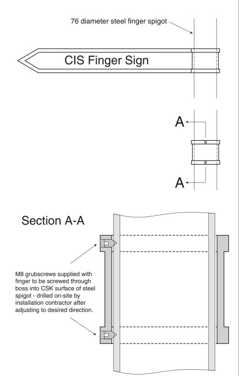
As standard a 1 - 1.5 metre length of plain galvanised tube is supplied with all finger posts. The fingers are to be sleeved over making sure spacer rings (if specified) are in place. Make an allowance for the finial and site cut the tube to the required length. Point fingers in the appropriate directions and tighten grub screws located to the rear of the boss.
