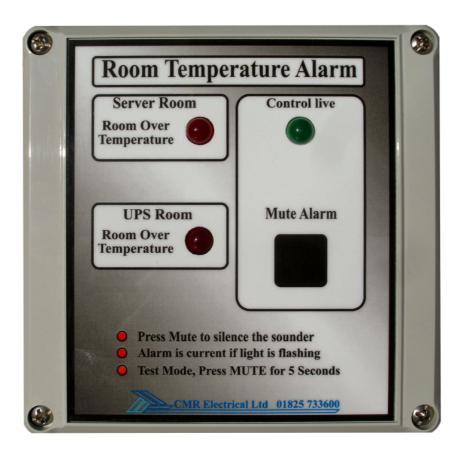
The RTA2 has been designed to monitor critical areas for high temperature via remote thermostats. Any number of thermostats can be connected to the control unit to give a common room over temperature alarm (RTA1) or two zones of temperature alarm (RTA2).
