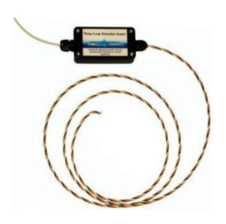
The unit has been designed to detect the presents of water or any conductive liquid. The RWM detects water by pulsing a bi-directional current (AC) across the sensors and closes a volt free relay contact when water is detected that can be used by existing alarm systems including Building Management Systems (BMS) or any existing alarm system such as a Fire alarm panel or burglar alarm.
