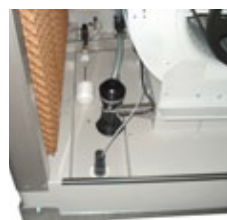
WATER FLOW REGULATION AND CONTINUOUS DRAINAGE SYSTEM, TO AVOID CONCENTRATION OF MINERAL SALTS.
