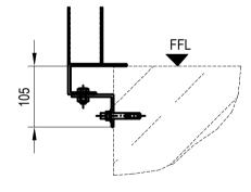
FIXING OF DOOR FRAME AT UPPER LEVELS
