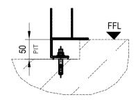
FIXING OF DOOR FRAME AT GROUND FLOOR LEVEL
