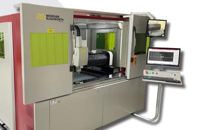
The Morgan Rushworth XL range of fibre lasers are equipped with an automatic shuttle table with dual pallet changer enabling parts to be safely loaded and unloaded whilst the machine is still cutting.
