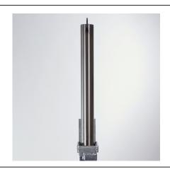
The RGP (removable ground post) offers a highly effective and robust way to protect premises and vehicles. The post is 500mm above ground, when removed the socket is covered using the integral lid. The post is lockable by rotating the post 45° and then pressing the high-security push button 7-pin security lock. The post is unlocked using the supplied key, rotated and then removed.
