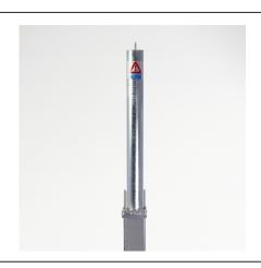
The RGP (removable ground post) offers a highly effective and robust way to protect premises and vehicles. The post is 900mm above ground, when removed the socket is covered using the integral lid. The post is lockable by rotating the post 45° and then pressing the high-security push button 7-pin security lock. The post is unlocked using the supplied key, rotated and then removed.
