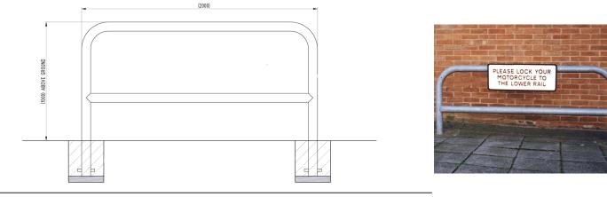
The Motorcycle Security Barrier is ideal for securing motorcycles. The Security Barrier is based upon a standard perimeter barrier of 76mm outside diameter tube, but has the addition of loose steel bars inserted into the lower horizontal tube and legs, this greatly increases the difficulty of cutting through the tube in order to make away with anything locked to the barrier. The Motorcycle Security Barrier is fully galvanised and only available in a Concrete in finish.
