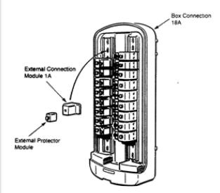
A BC 19A can also be fitted as the second DP on a pole where less than 10 dropwires are to be terminated and space is restricted, i.e. shared poles.
